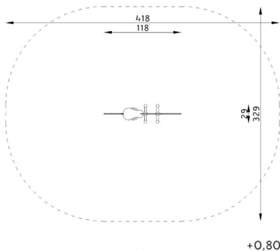
The device according to EN 1176-1:2012
