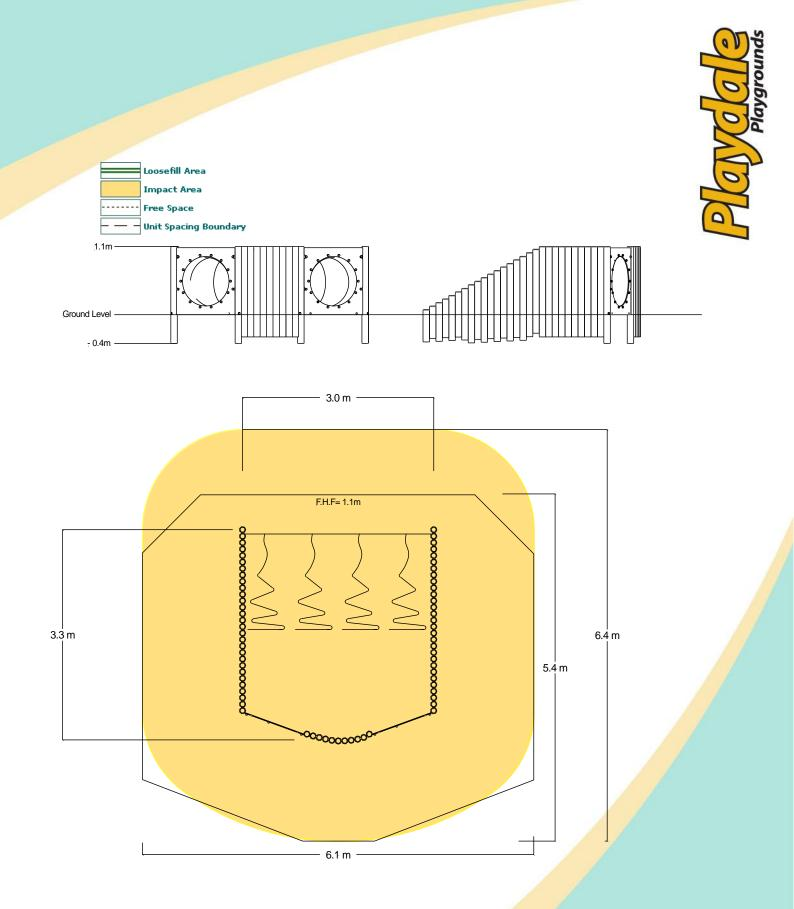
Note: These units are not suitable for use with Loosefill Surfacing.
