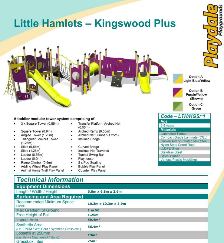
Surface Fixed Installation Information **Steel Ground Fixed** (if different) Installation Time 2 Person(s) 22 Hour(s) **Overall Weight** 813kg **Heaviest Part** 28kg Largest Part 2.4m x 0.5m x 0.5m Longest Part 2.4m **Concrete Required** 1.8m<sup>3</sup> Certified to EN 1176
