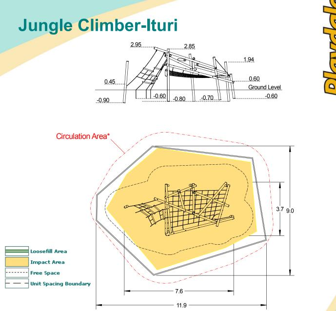
\* Recommended Circulation Area (1.2m outside impact area) – this area should be clear of solid raised objects (ie fences, walls, trees and other items of equipment). Loose fill retaining edgings are acceptable in this area.
